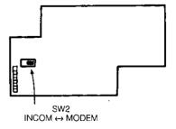
• When the product is shipped from the factory, each switch is set to the INCOM side or the HIGH side.
